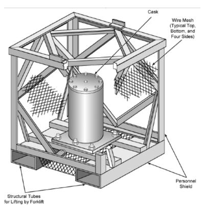
Figure 1: Schematic of the 9516 Type B package [3]
